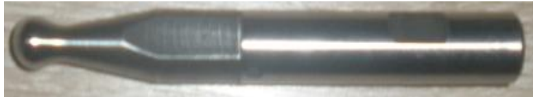
Fig. 2 – The tool which will be used at single point incremental sheet forming process.
